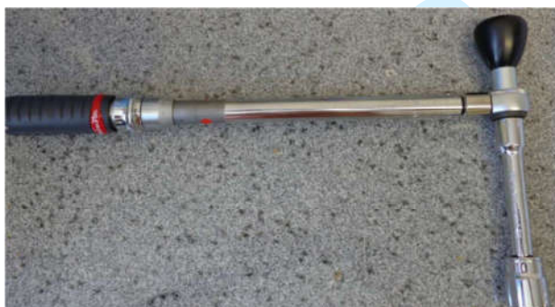
56 Figure 3. Torque wrench to close the autoclave. Source: Authors
