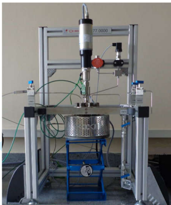
Figure 1. Frame with autoclave. Source: Authors
